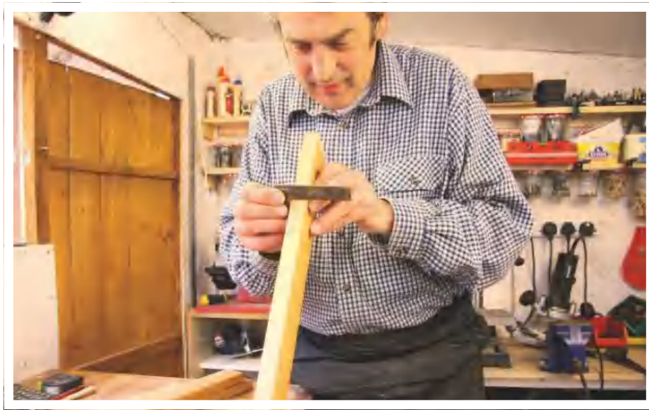
Squaring up a piece of beech for a coffee table
